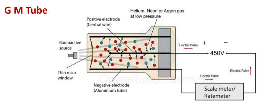
The tube contains argon gas at low pressure.
