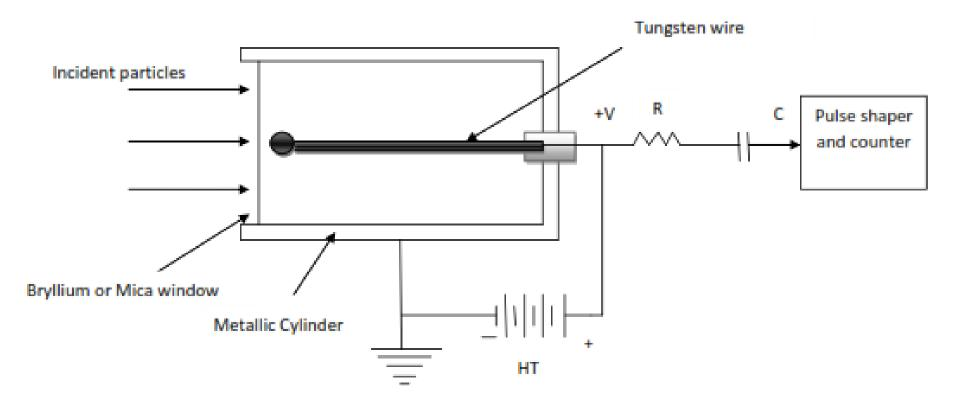
One of the electrodes is the outer metal cylinder connected to the – ve terminal of a dc-power supply and the other electrode is the central straight wire connected in series to a resistor R to the +ve terminal of the power supply (220 V).
