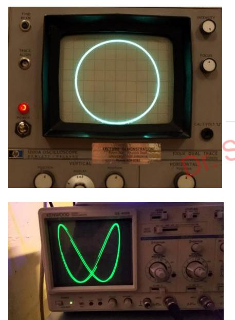
Two phase-shifted sinusoidal inputs are applied to the oscilloscope in X-Y mode and the phase relationship between the signals is presented as a Lissajous figure.
